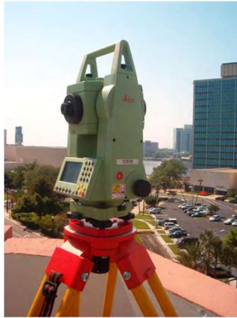
Figure 7: Leica TCR 705 Reflectorless Total Station.
