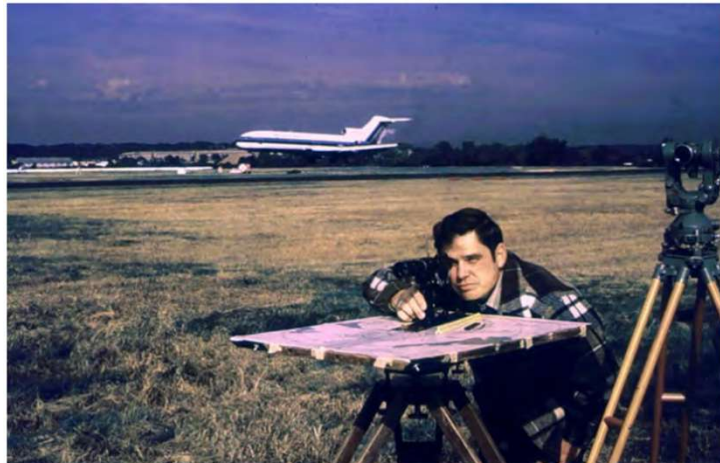
Figure 6: Plane table and alidade, Wild T-2 theodolite at right.
