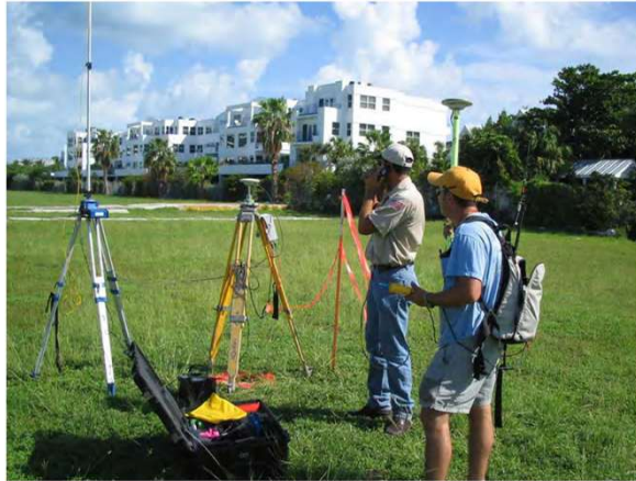
Figure 8: RTK base station and radio link transmitter, and rover with backpack.
