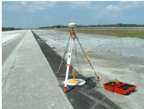
Figure 4: Airfield NAVAID positioning using Fast-Static GPS methods.
